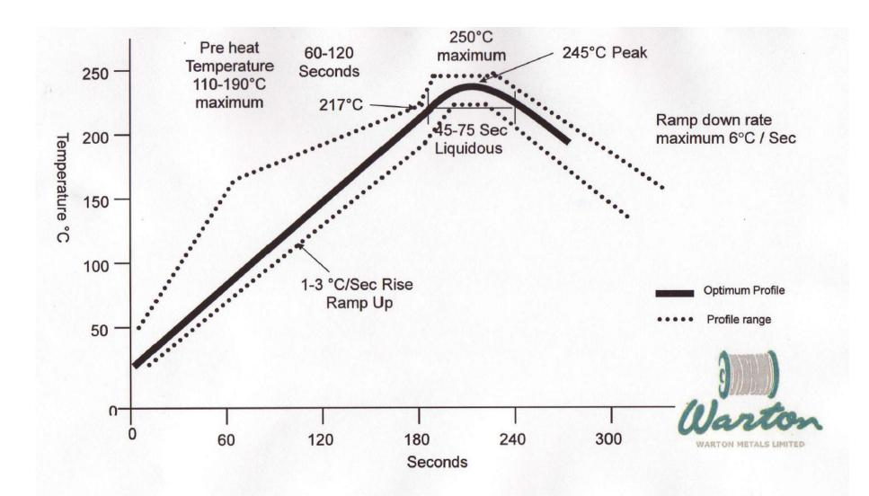
Microprint P2010 is suitable for Vapour Phase. The reflow profile for SnAgCu pastes using vapour phase reflow oven activation temperature range 140°C-170°C, peak temperature is 230°C-245°C,.
