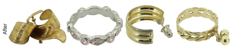
\* Samples cleaned in Ultrasonic cleaner model US-CU-CA-6L at 50 Degree's for 10 minutes.
